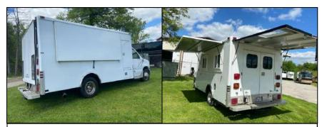
Awnings close to protect windows while in transit. Awnings open to reveal Rear door and (2) windows on either side of the coach allowing maximum exterior throughput of patients. The open awnings also provide patient weather protection at the windows.
