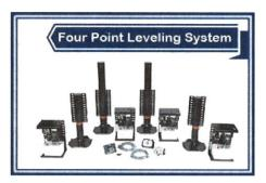
The difference between the Four Pump, Four Cylinder systems for the Class A Coaches is lifting capacity per jack.
